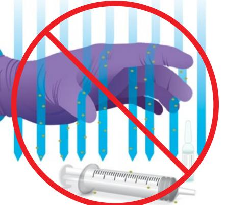
Personnel should never place hands above an object on the work surface. Contaminants from a user's hands may compromise the sterility of First-air (the undisrupted air coming directly from a HEPA filtration source).
