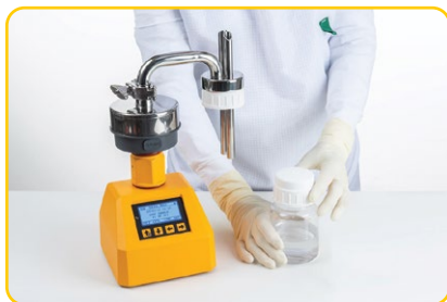
4. Connect the bottle with the collection liquid
