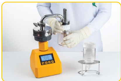
3. Disconnect the protective bottle
