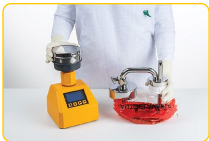
1. Remove the protective cover head from AIRBIO
